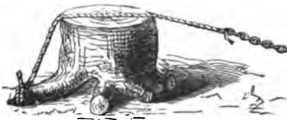
Fig. 145.—Removal of stumps by the forest-devil.
